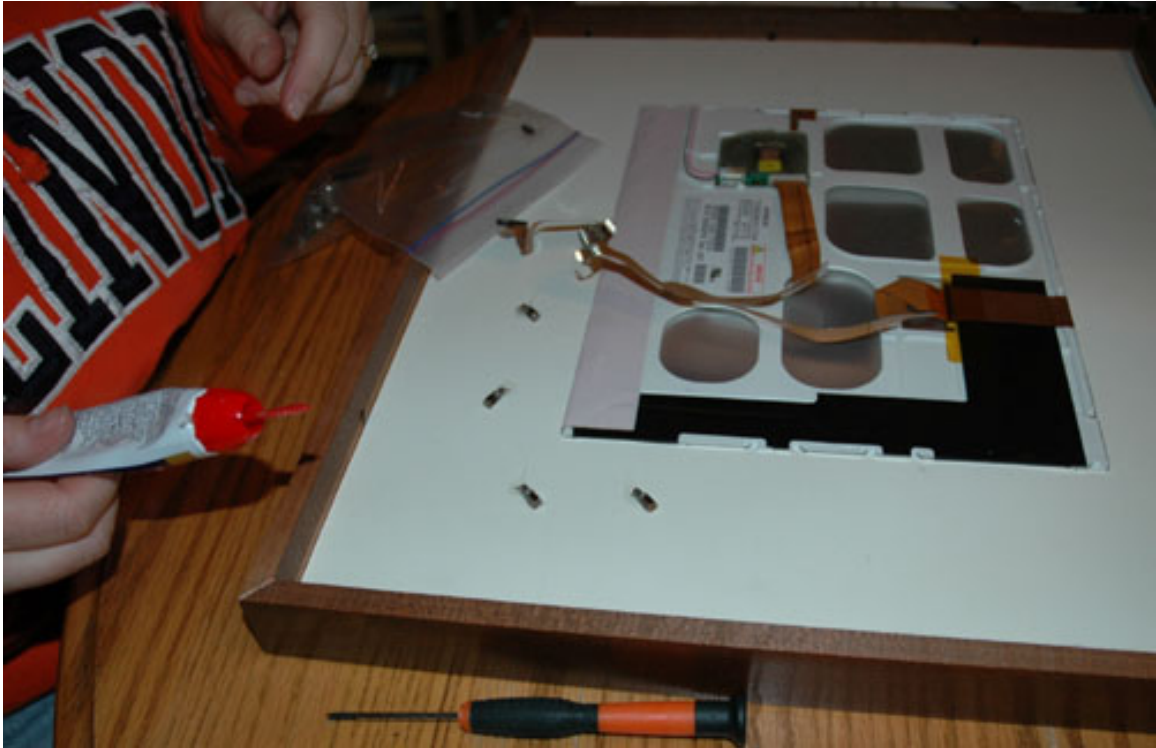
Here, the kick screw sockets are lying on their sides before being embedded into foam board.
